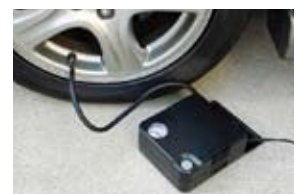
STEP2 | Fill up with air by air compressor
